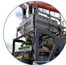
Aggregates loading system through rotating distributor
