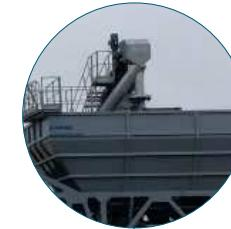
Aggregates loading system through reversible conveyor
